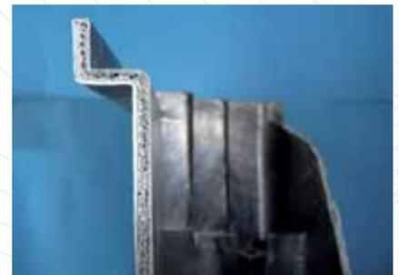
Thick, compact outer shell with foam for flexural rigidity
