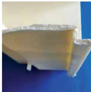
CELLMOULD® is a process developed by WITTMANN BATTENFELD to manufacture structured foam parts through direct gas injection with physical foaming agents. Structured foam components feature a compact shell with a foamed core. CELLMOULD® lightweight technology enables the production of extremely light, highly rigid parts without sink marks.
