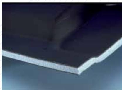
Compact surface with foamed core: shell and core made of one material or of different materials
