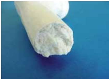
Fracture pattern of thick-walled part made of PBTGF 30, 66 % lighter
