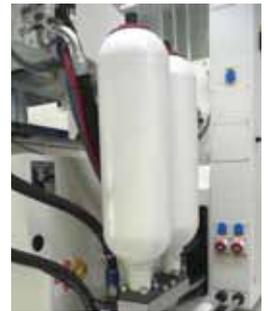
Optional hydraulic accumulator for high-speed injection
